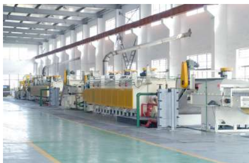
Continuous (Nitrogen Atmosphere Controlled) Heat Treatment Furnace, with process of De-phosphate and Carbon Potential Control 连续式热处理炉（氮气气氛保护） 配备有脱磷和碳势自动控制工艺
